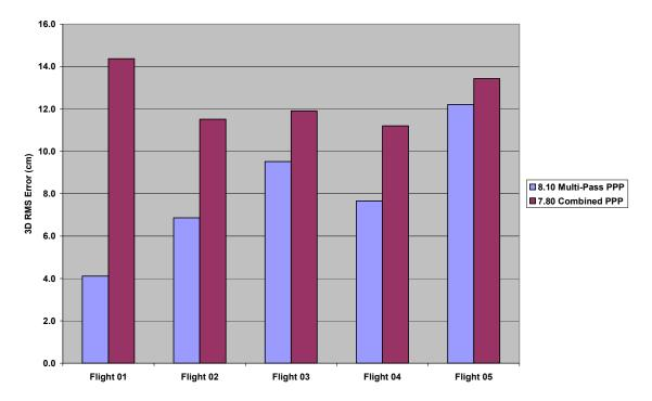
3D RMS PPP Accuracy Relative to a Differential Trajectory
